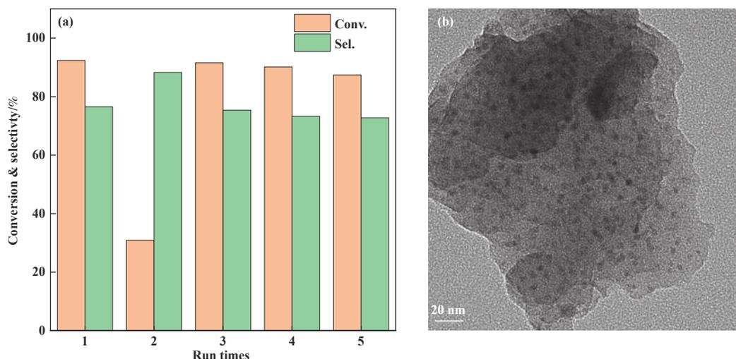
Fig.3 (a) Reusability test of Co/MNC-500 catalyst in hydrogenation of CyCONH<sub>2</sub>; (b) TEM pattern of reused Co/MNC-500 catalyst; Reaction condition: Co/MNC-500 50 mg, CPME 3 mL, CyCONH<sub>2</sub> 0.5 mmol, 180 °C, H<sub>2</sub> 3.0 MPa, 12 h
