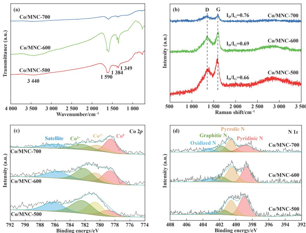
Fig.2 (a) FT-IR spectra; (b) Raman spectra; (c) Co 2p; (d) N 1s spectra of Co/MNC-500, Co/MNC-600 and Co/MNC-700
