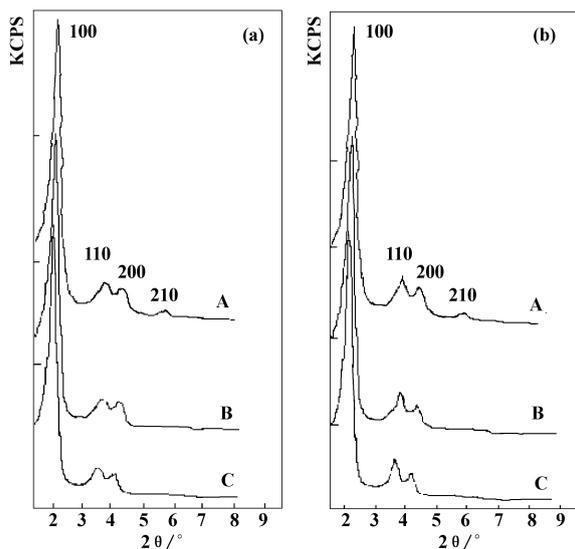
Fig. 2 Low angle XRD patterns of (a) dried samples (A, B and C); (b) calcined samples (A, B and C)
