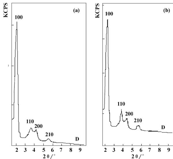
Fig. 3 Low angle XRD patterns of (a) dried sample D; (b) calcined samples D
