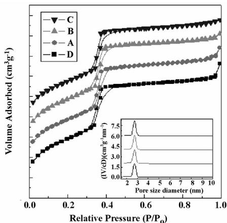
Fig. 4  $N_2$  adsorption/desorption isotherms and pore size distribution from desorption branch of samples A, B, C and D obtained by a Micromeritics TriStar 3000 analyzer at 77 K. Isotherms of A, B and C have been offset by 100, 200 and 300  $\text{cm}^3\text{g}^{-1}$  along the vertical axis for clarity, respectively.
